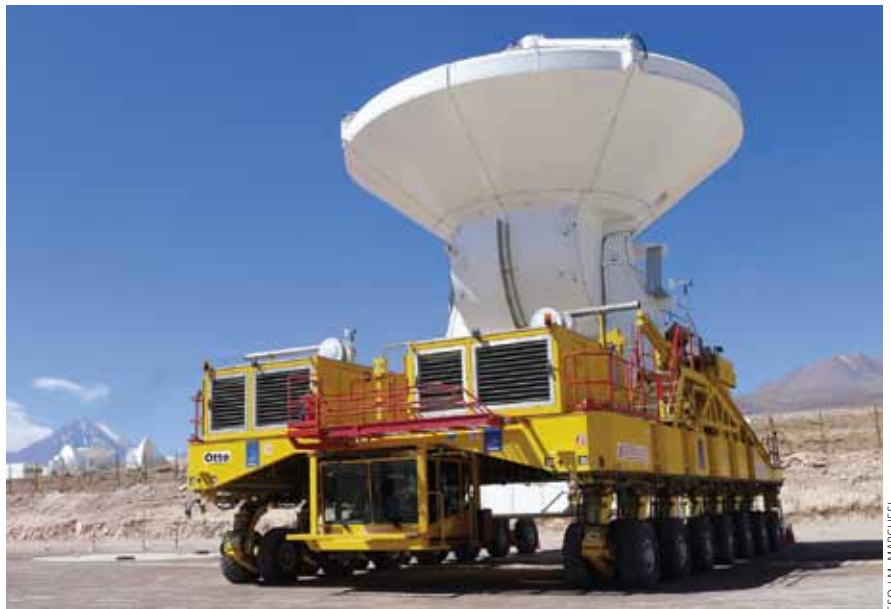
ROLLING OUT THE ANTENNAS Left: When astronomers want to change the configuration of the 66 antennas that make up the Atacama Large Millimeter/submillimeter Array (ALMA), they don’t do it by hitting a button: transporter operators move the antennas for them. Here, Patricio Saavedra drives the 28-wheel transporter “Otto” across the ALMA site — while wearing an oxygen tube to keep his mind sharp at an elevation of 5,000 meters. Right: Here, Otto carries the array’s final 12-meter antenna, delivered to ALMA in 2013. The driver’s cab is the box in front. The antenna weighs about 100 tons.
