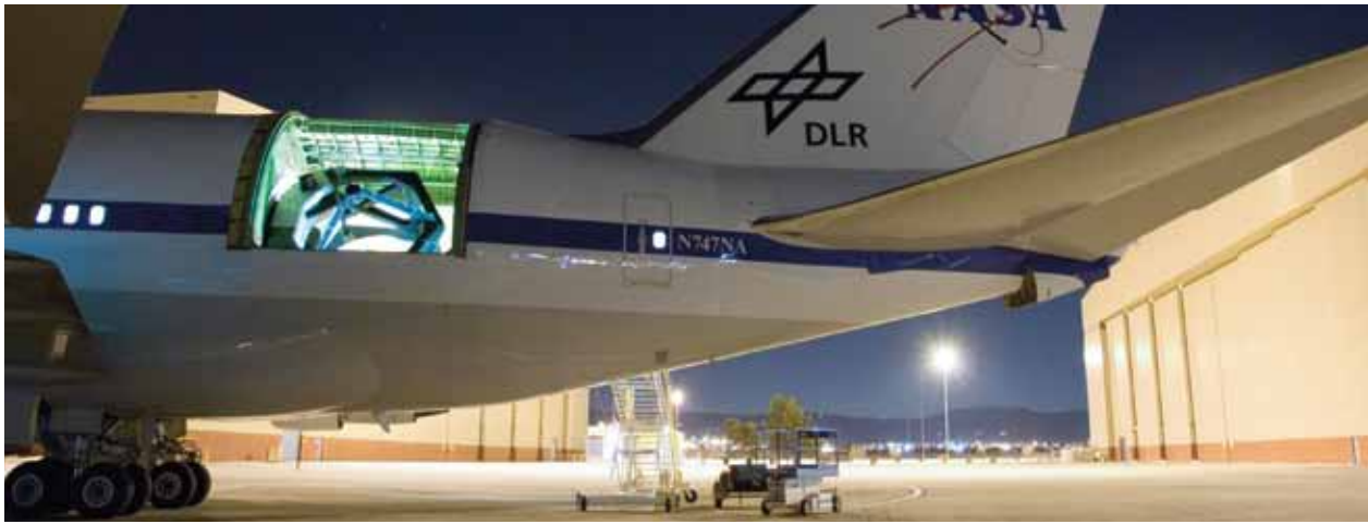
OVERSIZED CARRY-ON SOFIA is a modified Boeing 747 that flies high above the atmospheric water vapor that interferes with ground-based telescopes. Its 2.5-meter reflecting telescope peeks out from the rear fuselage.
