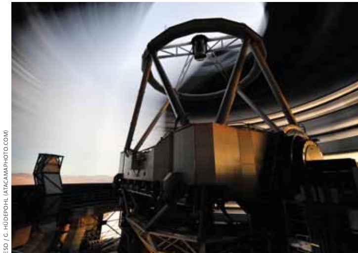
NIGHT CLASSES Left: One of the 8.2-meter telescopes of the four-scope Very Large Telescope at Paranal, Chile. Right: Telescope instrument operator Claudia Cid (left) gives data-handling administrator Cecilia Cerón a crash course on how TOs prepare for the night's observations, while sitting in the Very Large Telescope's control room. Cerón and her colleagues oversee the observatory's data flow, beginning when the instrument takes an image in Chile and ending when it's delivered to ESO staff in Germany.
